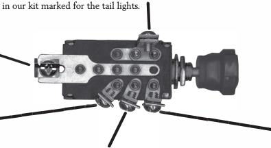
Low Beams: runs from the head light switch to the low beam terminal on both head lights using 14 gauge wire. This wire will have 12 volts when the head light knob is pulled out to the third position. This will be the red wire in our kit.
