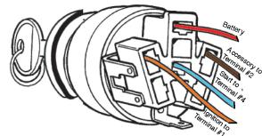
WIRING: Engraved in the black plastic area on the base of the switch is abbreviated wording defining each spade terminal. Follow the chart below for the proper connections to the switch.
