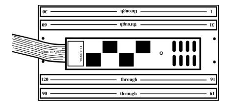
**Bag #40A MASS AIR FLOW SENSOR including INTAKE AIR TEMPERATURE (MAF):** On a factory installation, this sensor is mounted in the intake air duct between the air cleaner and throttle body. Plug the five gang black connector into the sensor and run the wires back to the panel. Connect the Tan wire MAF A->3 to #3, the Purple wire MAF B->2 to #2, the Black wire MAF C->30 to #30, the Pink wire MAF D>24 to #24 and the Yellow wire MAF E->1 to #1.
